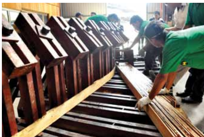
The flexible characteristic of glulam is important to produce curved glulam members.
