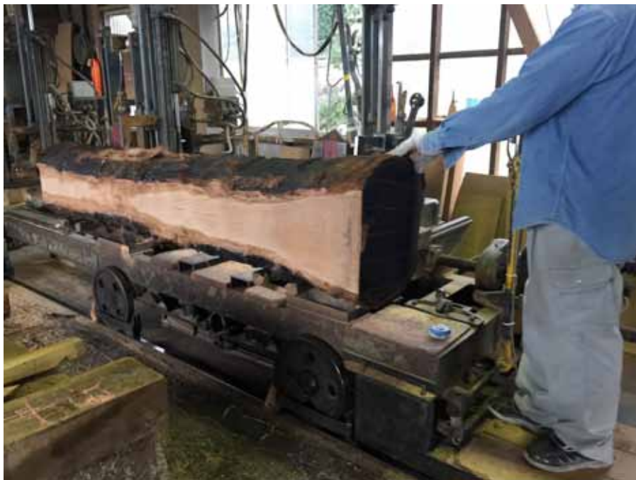
Sawing for the treated OPT log.
