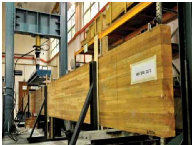
Straight Mengkulang beam, undergoing load bearing test.
