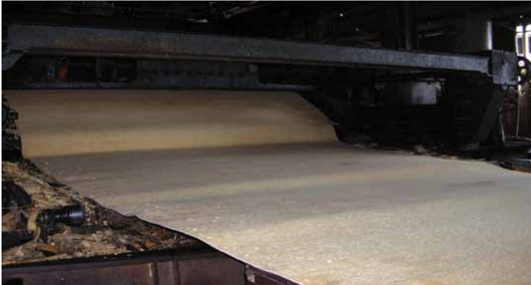
The peeling process is undertaken at the rotary lathe and spindle-less lathe, converting the OPT logs into thin sheets of veneer.
