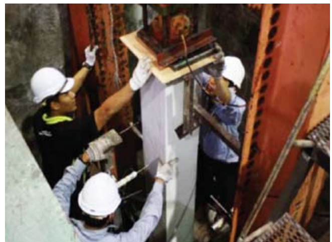
Pillar box installation and compression test in the laboratory of the Faculty of Civil Engineering, UiTM.
