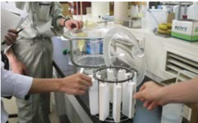
Samples being tested for formaldehyde emission test at the Japan Testing Centre for Construction Material in Saitama.
