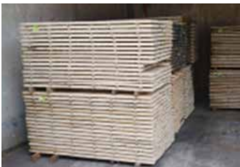
Oil palm timber charged into a kiln chamber.
