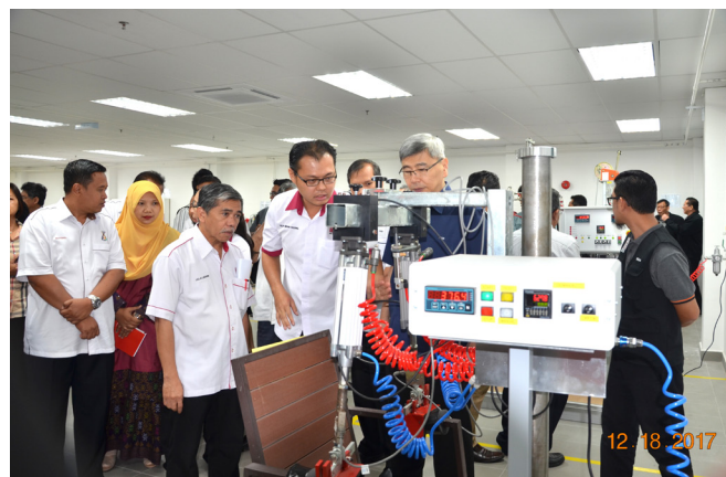
Demonstration on the armrest durability testing machine.
