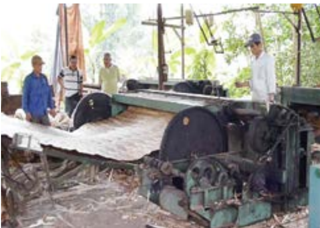
Log peeling in progress.
