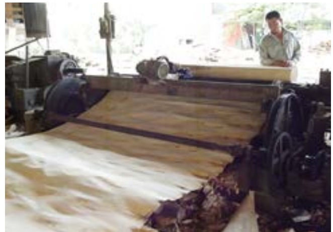
Log peeling in progress.
