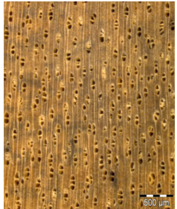
Figure 2: Macroscopic Structure Of N. cadamba (kelempayan/laran)(10 ×)
